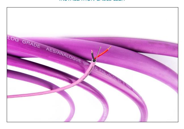
Van Damme Purple Series Digilog Ecoflex is a Low Smoke Zero Halogen (LSZH) jacketed audio multicore specifically for installation use. The use of LSZH cables is becoming a specified essential in public buildings and new build construction projects. Based electrically and mechanically on the Van Damme Green Series range this cable will carry AES/EBU and/or analogue balanced audio as well as paired data signals such as RS485, RS422 and DMX512.
