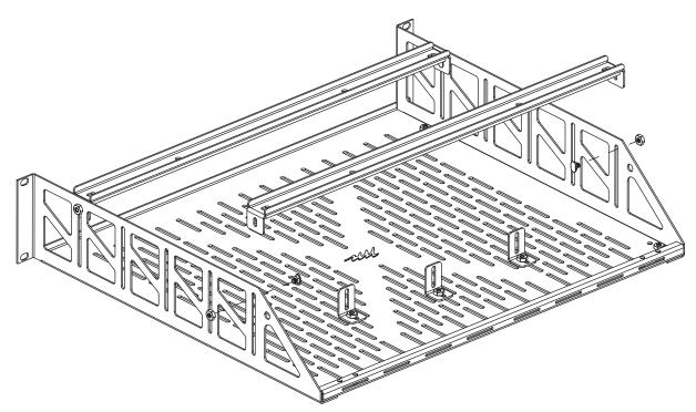
Three (3) Rear Brackets are provided to prevent unit from sliding back. (Here are four ways brackets can be mounted)
