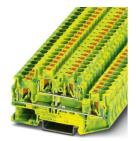
Protective conductor double-level terminal block, connection method: Push-in connection, 1st and 2nd level, cross section: 0.2 mm<sup>2</sup> - 6 mm<sup>2</sup>, mounting type: NS 35/7,5, NS 35/15, color: green-yellow
